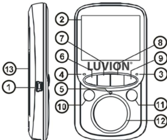
1. **Power connector** - Connect the included USB power adapter to power and/or charge the parent unit.
